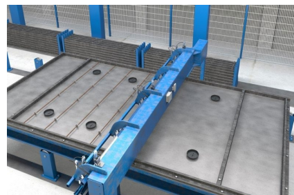
Reinforcement is placed by a transverse iron machine.
