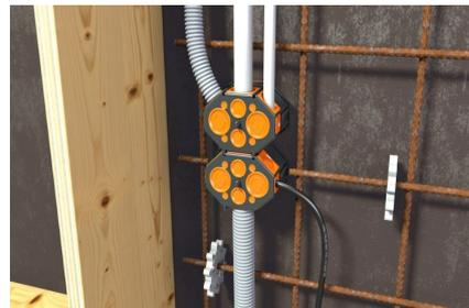
Insert cables or pipes M20/25/M32. Membrane technology enables an absolutely concrete-tight insertion
