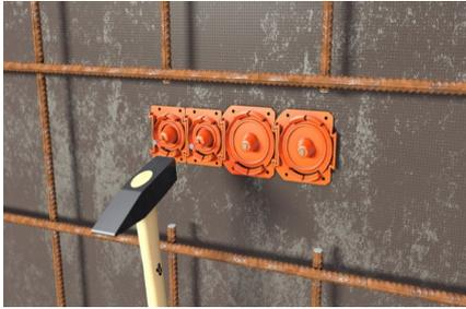
Wall mounting: Nail front part to formwork. Integrated nail fixation enables easy assembly. The front part can be firmly connected to other manifolds by means of the plug-in system.
