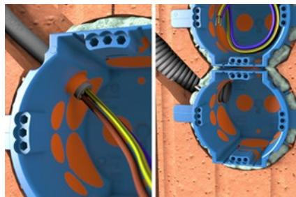
Simply push cable through Cable-Plopp or open diaphragm with cutter knife and insert tubes.
