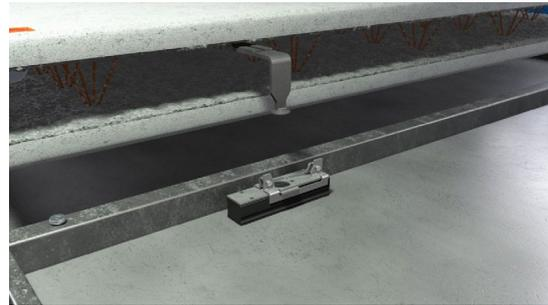
Double wall is lifted, magnet remains on the switching table.
