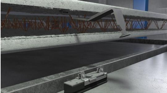
The sword is pulled out of the cap set in concrete.
