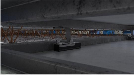
Magnets fix the first concrete shell to the second formwork table.
