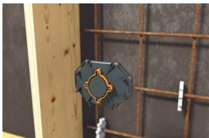
Cover is particularly suitable for luminaires with narrow luminaire base due to 35mm opening.
