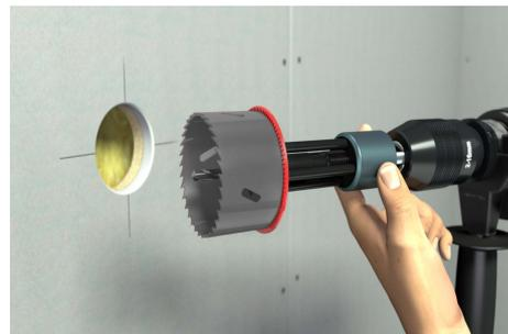
Hold the aluminum sleeve and return the adapter to the starting position by turning the drill clockwise.
