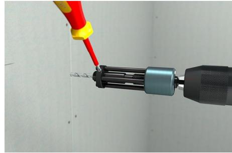
Fix the centering drill with fixing screw on the side.
