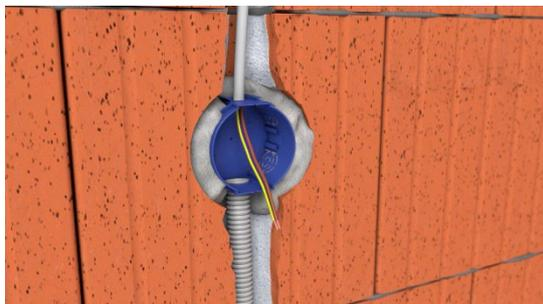
Mill the drill hole for the base of the box. Set the bottom part of the box flush, insert the cables and pipes.
